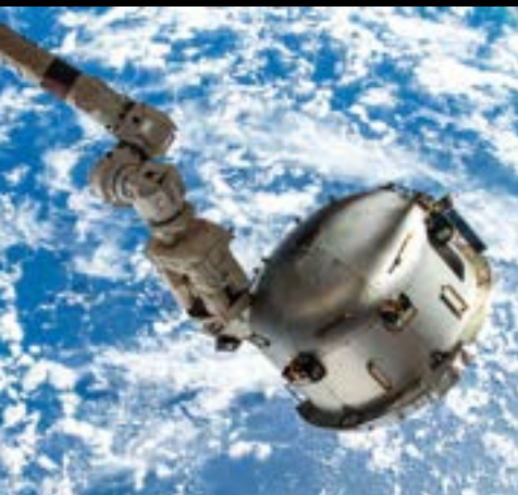
📍 264 miles (425 kilometers) above the Atlantic Ocean off the coast of southern Brazil, the Nanoracks Bishop airlock is seen attached to the Canadarm2 robotic arm's latching end effector. Bishop can be uninstalled from its home on the Tranquility module for portable operations and can also be used to stow cargo and extract or install payloads.
