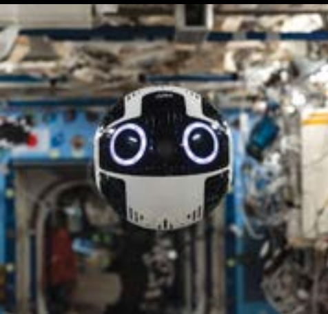
JAXA's (Japan Aerospace Exploration Agency) free-flying robotic camera performs a technology demonstration inside the Kibo laboratory module. It is being tested for its ability to autonomously maneuver and navigate aboard station while photographing and videotaping crew activities.
