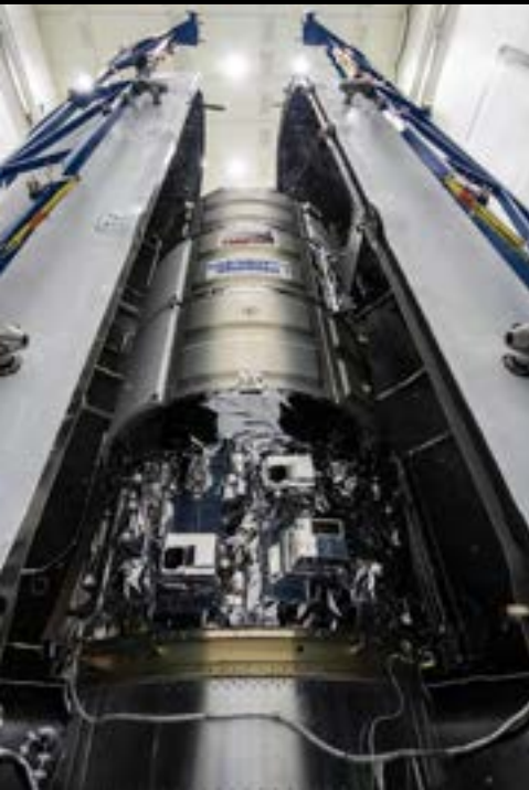
The Northrop Grumman Cygnus resupply spacecraft is seen being encapsulated inside the SpaceX Falcon 9 payload fairing as it prepares to launch from Space Launch Complex 40 at Cape Canaveral Space Force Station in Florida. The 20th Northrop Grumman commercial resupply service to the space station supported the Expedition 70 crew.
